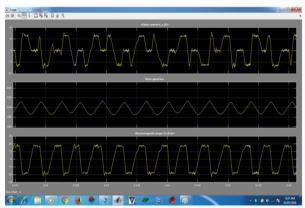
Fig.11 Output waveform of the stator current, speed and torque of the motor
