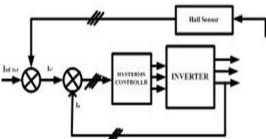
Fig.4 Block dia of hysteresis current controller
