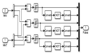
Fig.5 Simulink model of hysteresis current controller
