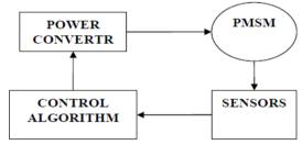
Fig.1 Block Diagram of Bldc motor control
